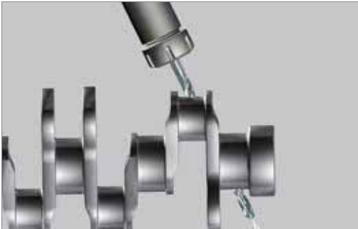
Oil Bore - Mach Long Drill(MLDA)
