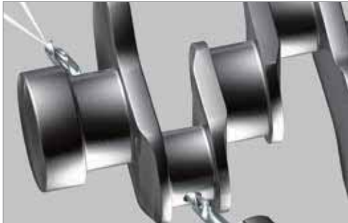
Oil Bore - Mach Long Drill(MLDA)
