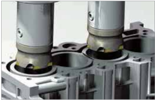
Cylinder Bore(Roughing) - Boring Cutter
