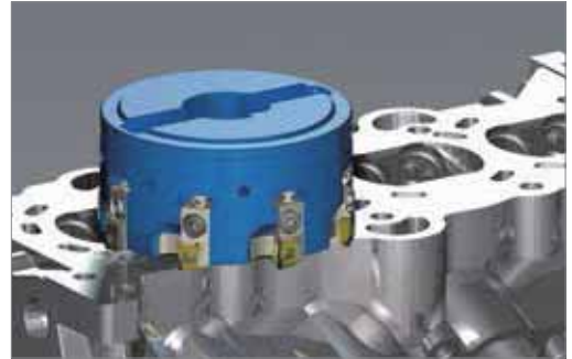
Top Face(Roughing & Finishing) - Aero Mill
