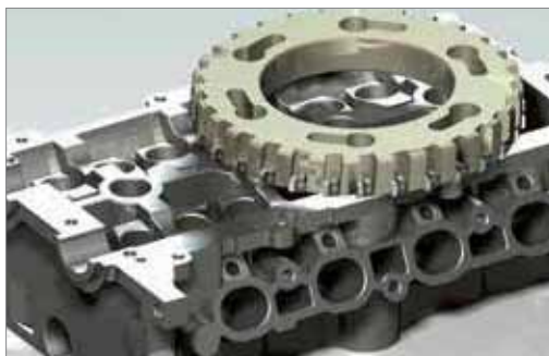
Bottom Face(Roughing & Finishing) - High feed Cutter
