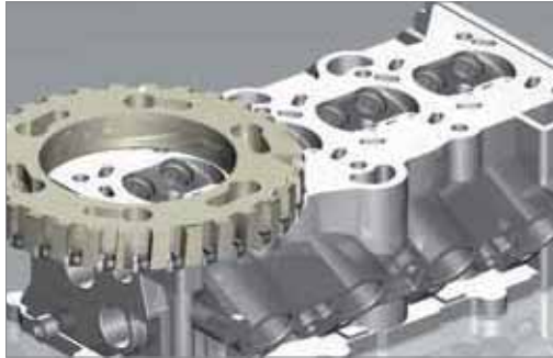
Top Face(Roughing & Finishing) - High Feed Cutter
