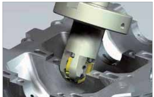
Crank Bore(Crankshaft Bearing Bore) - Form Cutter
